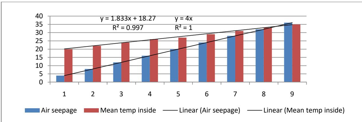
Fig. 2: The relation between air seepage and mean temperature
